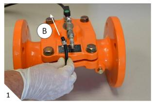
2. Using a 16mm spanner, disconnect the control tube from the restriction orifice [C] - [D].
