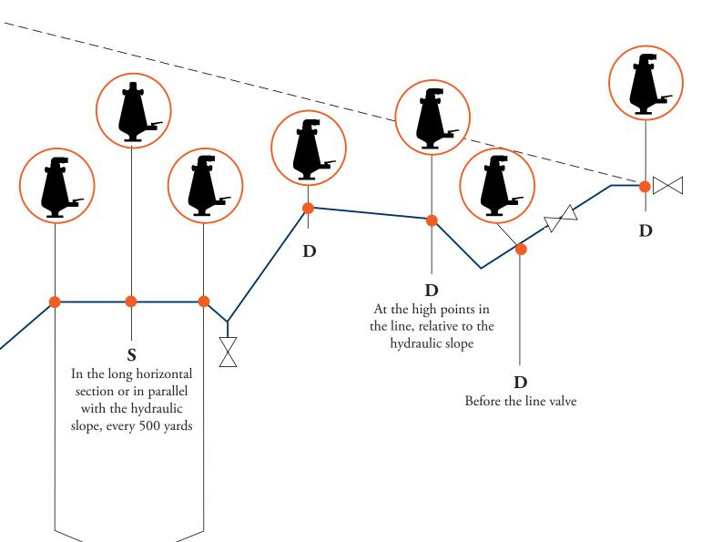
At the dropping ends of the horizontal section or in parallel with the hydraulic slope.
