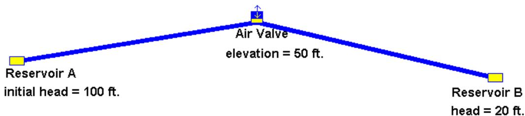
Simple transient flow model to calculate “Air Slam”
