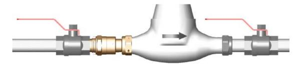
Figure 2 – Connection of **UFR** with union nut connection, upstream of the water meter.
