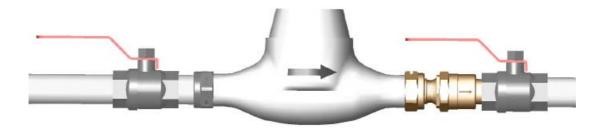
Figure 1 Connection of **UFR** with union nut connection, downstream of the water meter.
