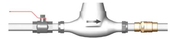
Figure 3 – Connection of **UFR** with threaded male or female connections, downstream of the water meter.
