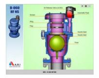
The three-stage non-slam air valve is equipped with an additional disc that has a small orifice (but much larger then the automatic orifice). The air valve is normally open with a large active orifice. The large discharge
