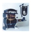
Two-stage non-slam air valves are actually a vacuum breaker with a smaller (automatic) air release orifice and larger air intake orifice. The discharge orifice is held in place by a spring so that it is normally closed. Thus, the air valve can only release air through the small orifice. When a vacuum condition occurs in the pipeline (water is draining out of the pipe, at water column separation), the check valve disc opens, allowing for the intake of air through the larger orifice.
