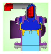
The Dynamic air valve operates in a totally different manner. It discharges all the air in the pipeline through the large orifice when the water column arrives and closes the air valve slow enough to prevent an abrupt change of velocity. This action prevents surge and water hammer. The unique rolling diaphragm sealing mechanism reduces changes in velocity (in equation  $\Delta H = (c/g) \Delta V$ ), therefore reduces the slam effect.
